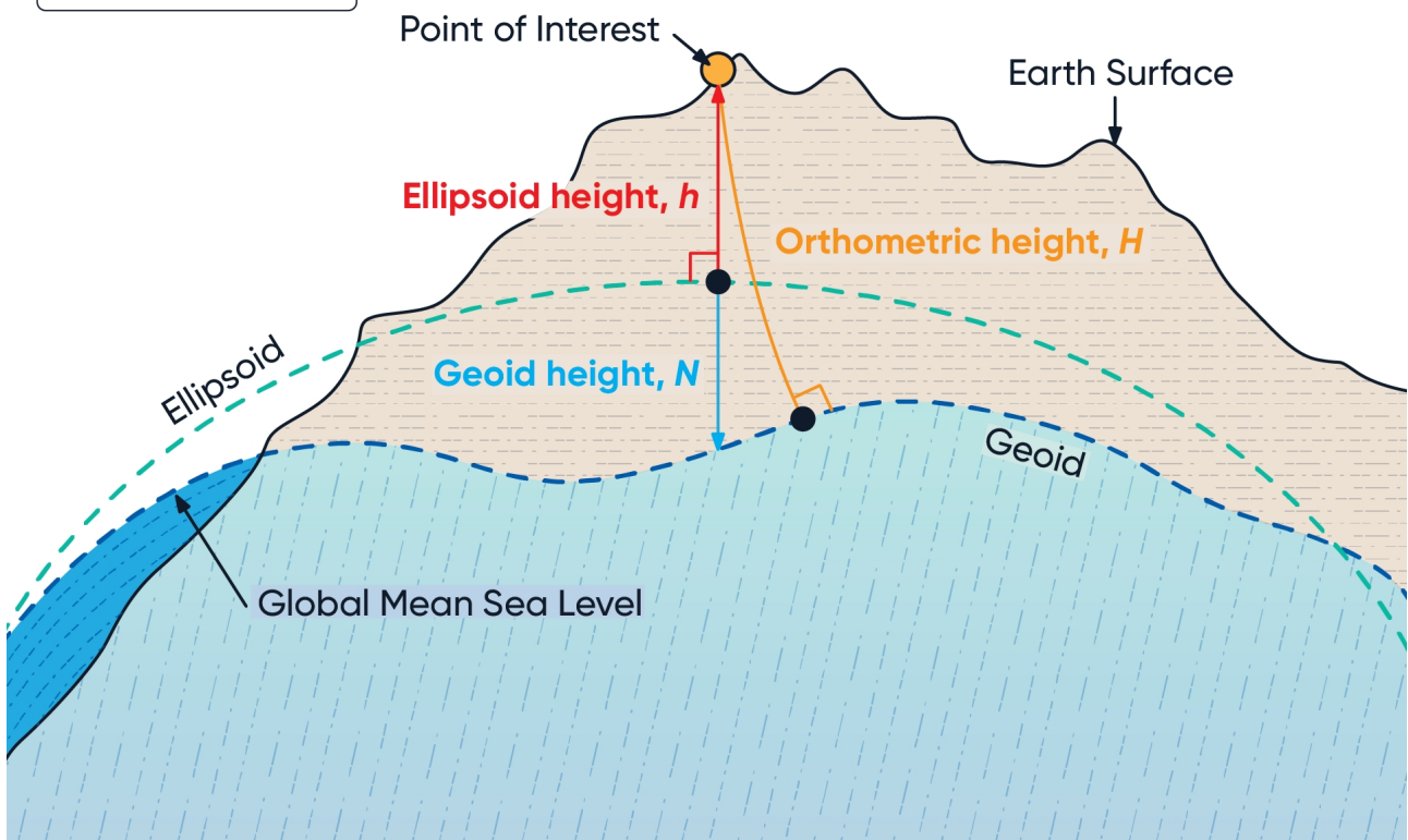
Figure 62: Orthometric, ellipsoid and geoid height diagram
