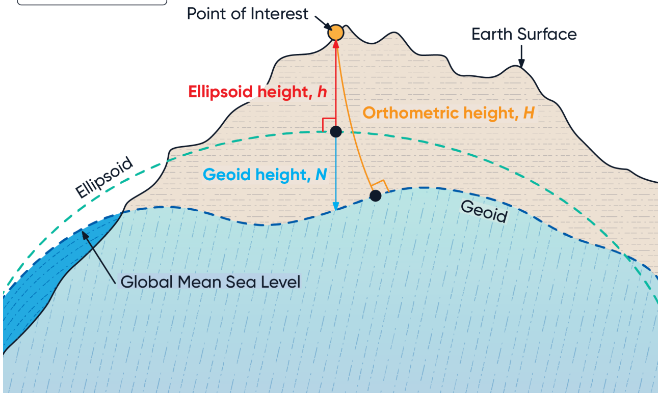
Figure 94: Orthometric, ellipsoid and geoid height diagram
