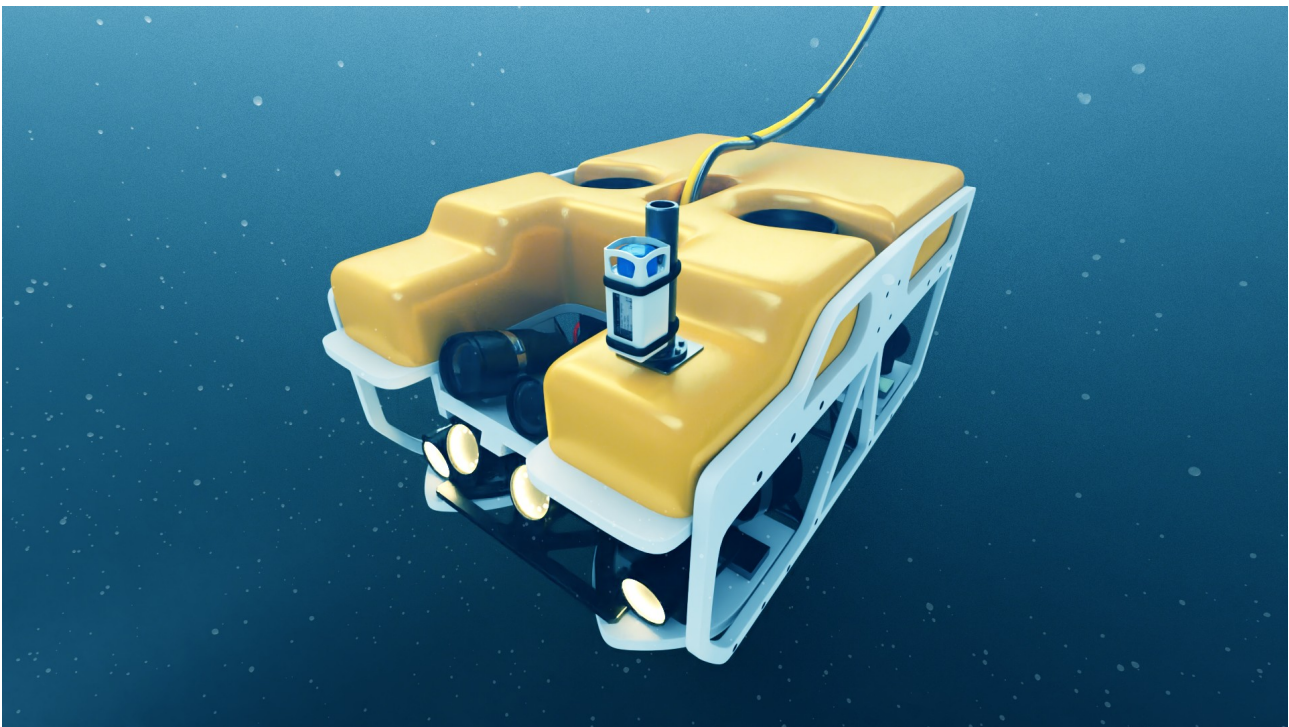
Illustration 8: Example Subsonus Tag Mounting
