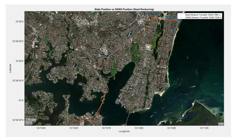
At the end of the test, Certus' dead reckoning position was compared with the GNSS reference position and the error was found to be just 105.2 metres or 1.0% of distance travelled. The position error over time and final approach can be seen below comparing the Certus position output with the GNSS reference position.
